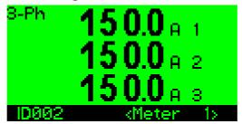
This page shows measured values from the selected meter/load. This data is meaningless for an unconfigured **multicube** system as the programmed Current Transducers may not match the physical devices fitted.
