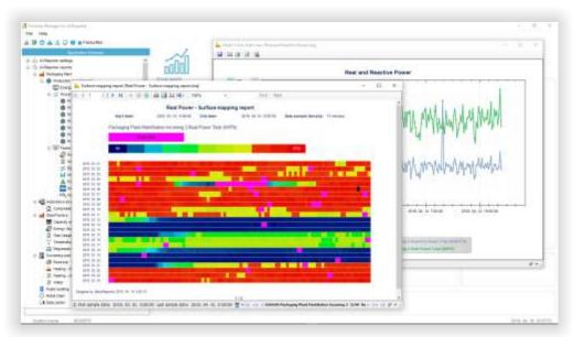
Surface mapping - monitoring the utilisation of production lines
